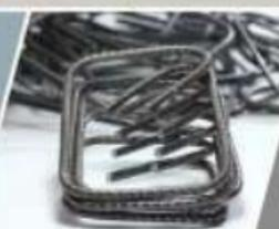
Profile on shape and size, anti seismic loop - min 75 mm with 135° bending as per standard. Angle bend with radius as per standard.
